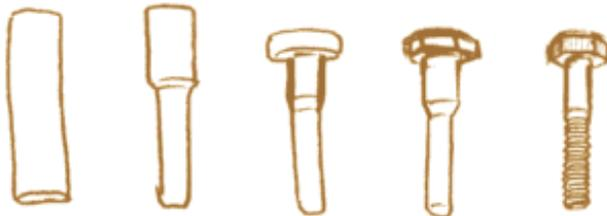
**COLD HEADING/COLD FORGING**
