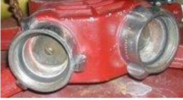
this siamese clapper inlet allows one or two inputs into a deluge gun.
