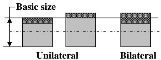
**Fig. 1.3.2 Types of tolerance**
