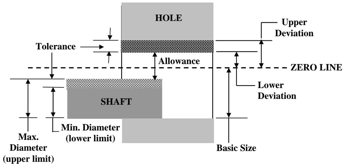
**Fig. 1.3.1 Interrelationship between tolerances and limits**
