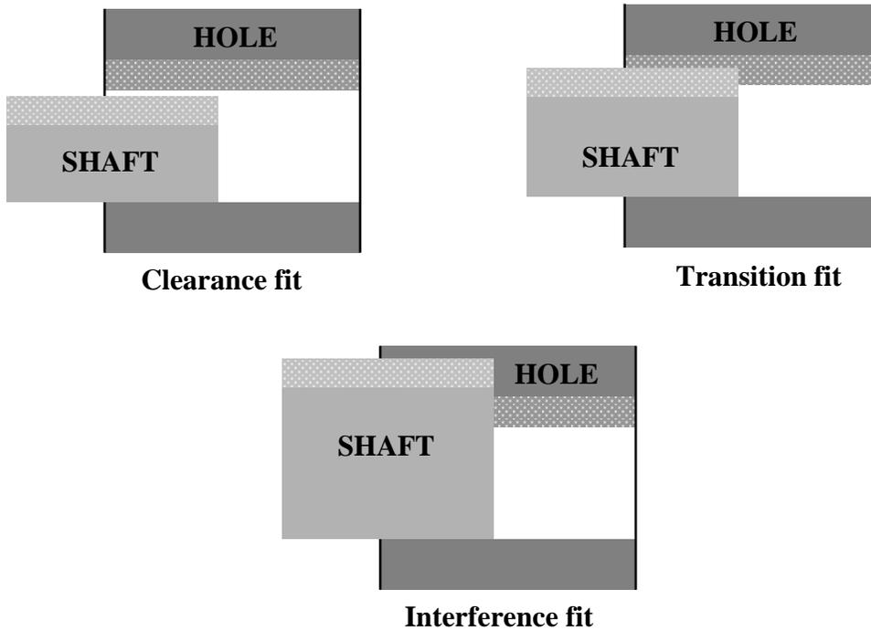
**Fig. 1.3.3 Schematic view of Fit system**
