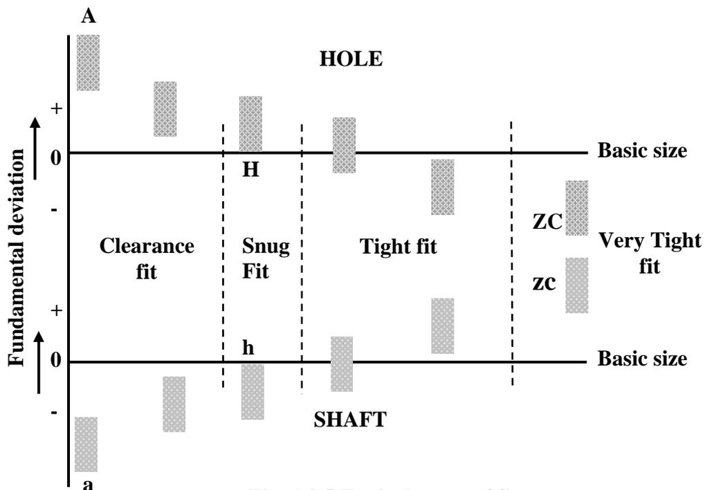
**Fig. 1.3.5 Typical zones of fit**
