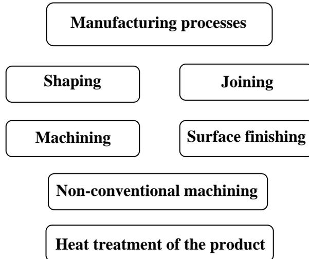
**Fig. 1.3.6 Common manufacturing processes**
