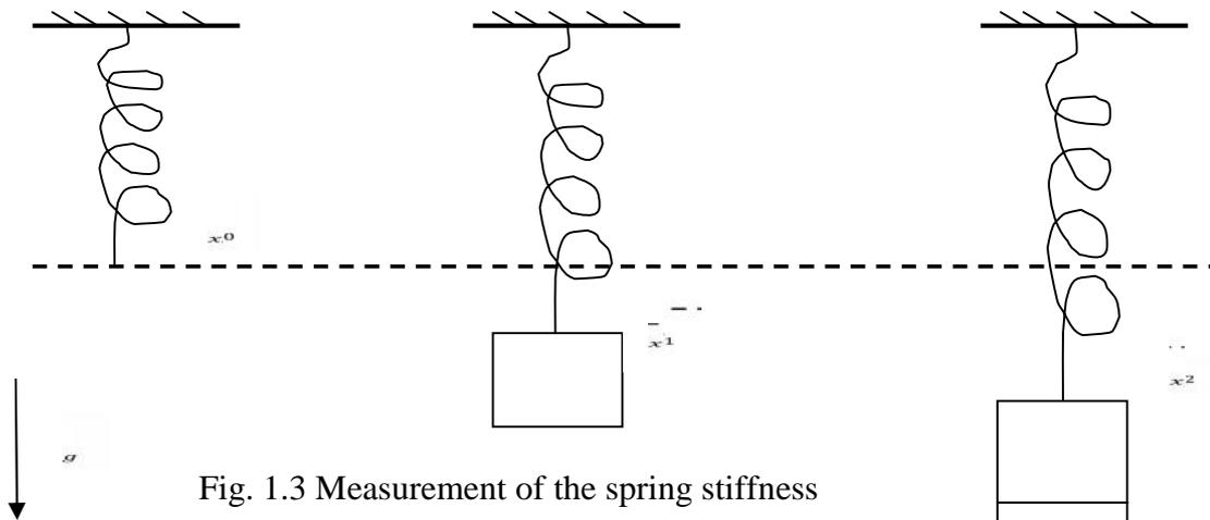
Fig. 1.3 Measurement of the spring stiffness
