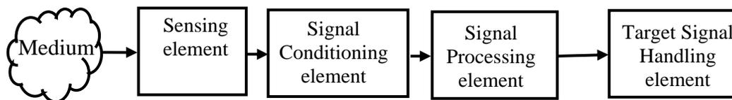
**Fig. 2.1 Functional configuration of a typical sensor system**
