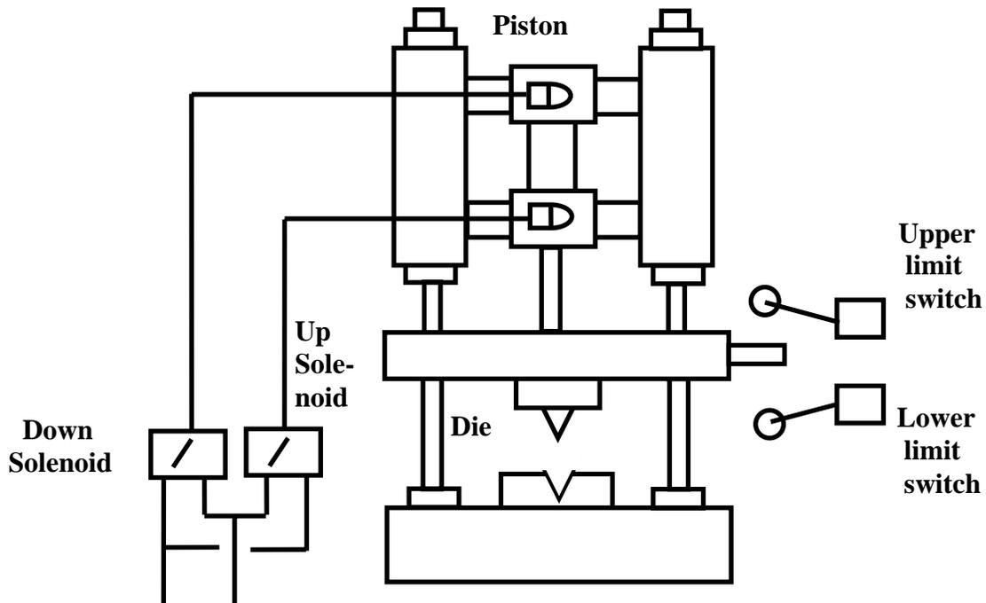
The control computer for the process has 3 inputs (2 from the limit sensors and 1 from the master switch) and controls 2 outputs (1 to each actuator solenoid).
