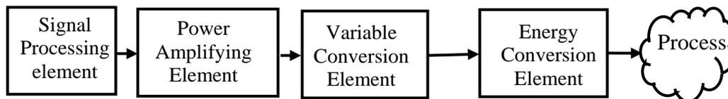
**Fig. 2.2 Functional configuration of a typical actuator system**
