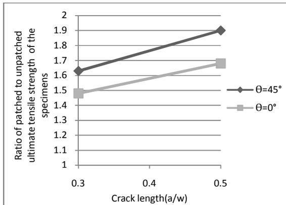
Fig. 7 Comparison of increment of ultimate load of specimens with different crack length, repaired by F-A-F patch
