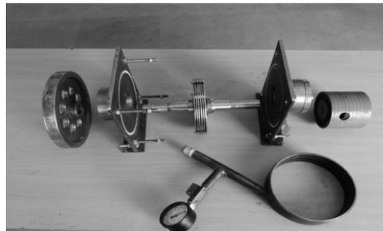
Fig. 2 : Parts of Multiple disc Turbine.
