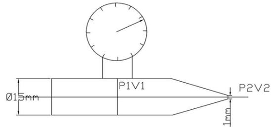
Fig. 1 : Nozzle Arrangement - line diagram for Test Rig
