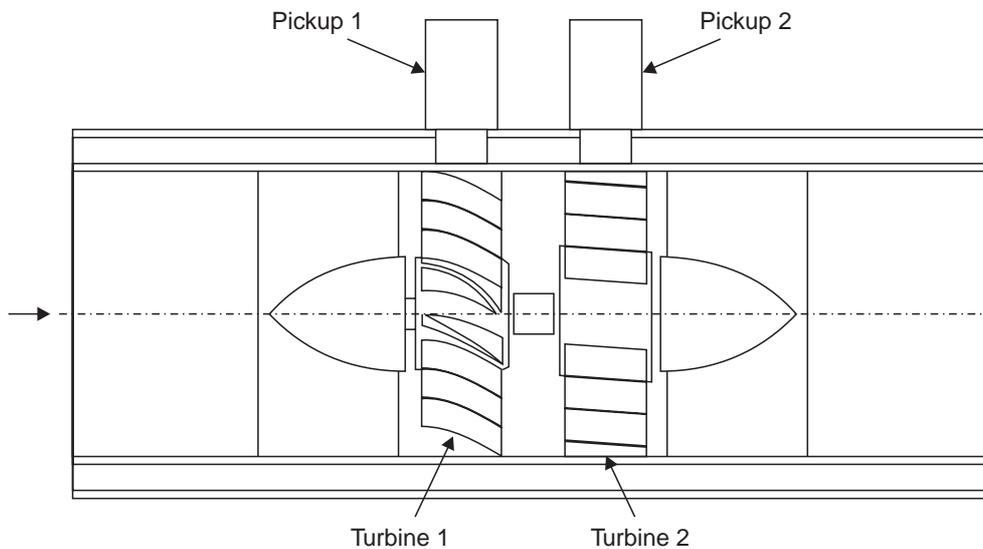
**Fig. 1.41** Twin-turbine mass flow meter
