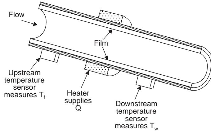
**Fig. 1.46** Thermal flow meter with external elements and heater
