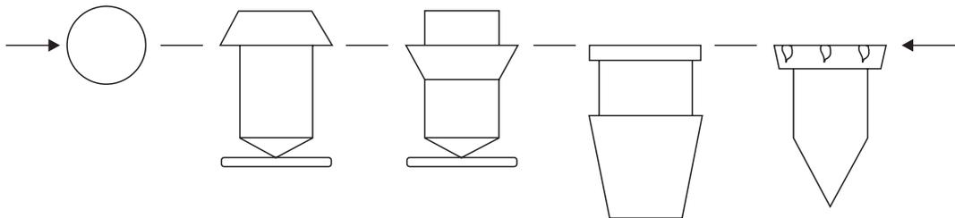
**Fig. 1.38** Partial representation of typical rotameter float shapes
