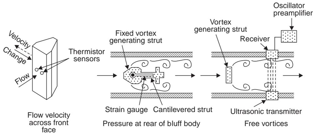
Fig. 1.71 Solid state vortex flow meter detectors
