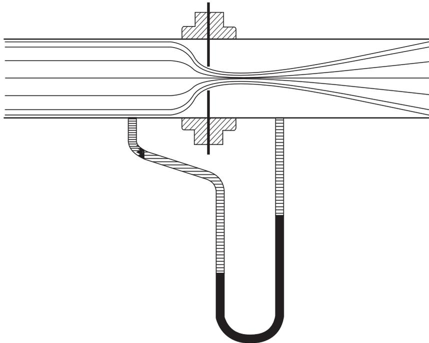
**Fig. 1.2** Orifice and Pressure-Differential Measurement
