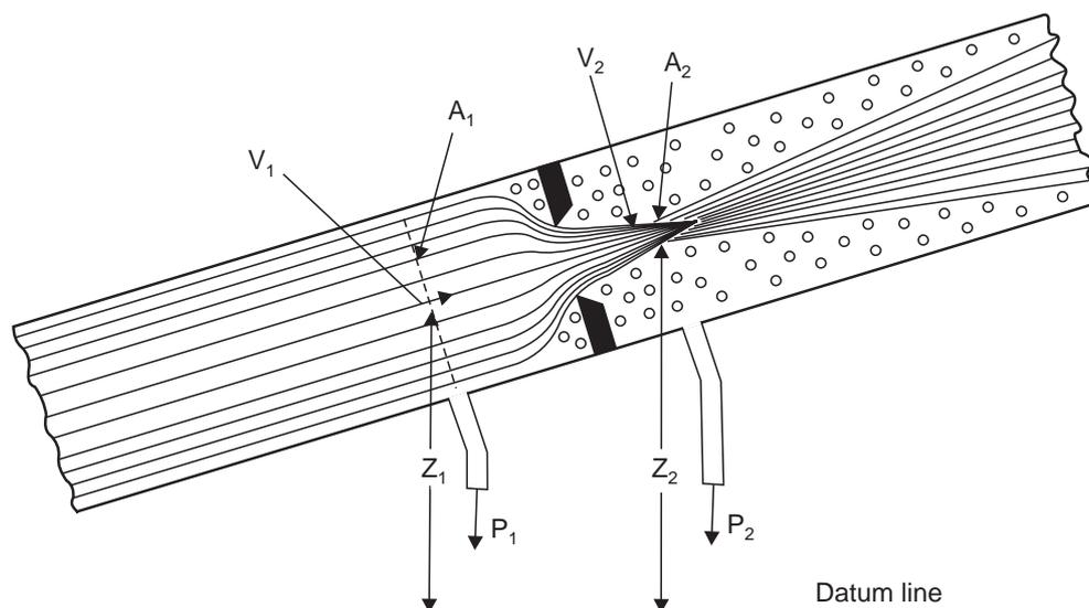
Fig. 1.1 Schematic representation of a one dimensional flow system with a restriction
