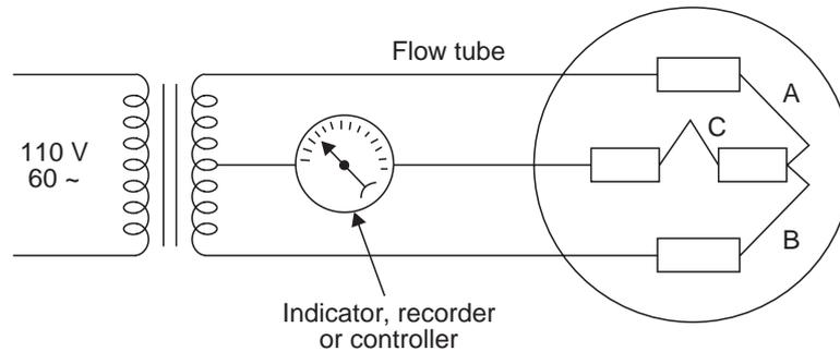
Fig. 1.49 Hot wire flow-sensing probe
