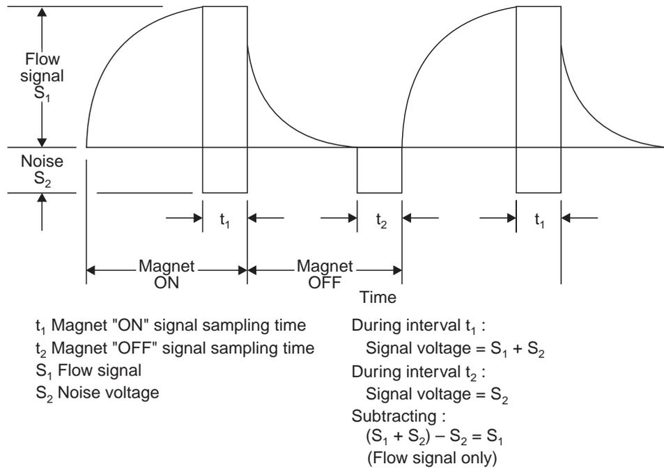
Fig. 1.54 Plot of the output signal
