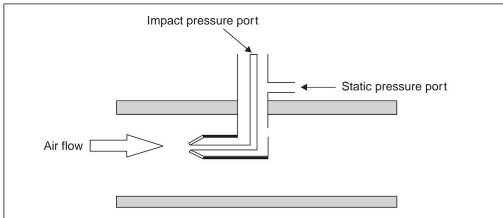
Fig. 1.21 A common industrial type pitot tube
