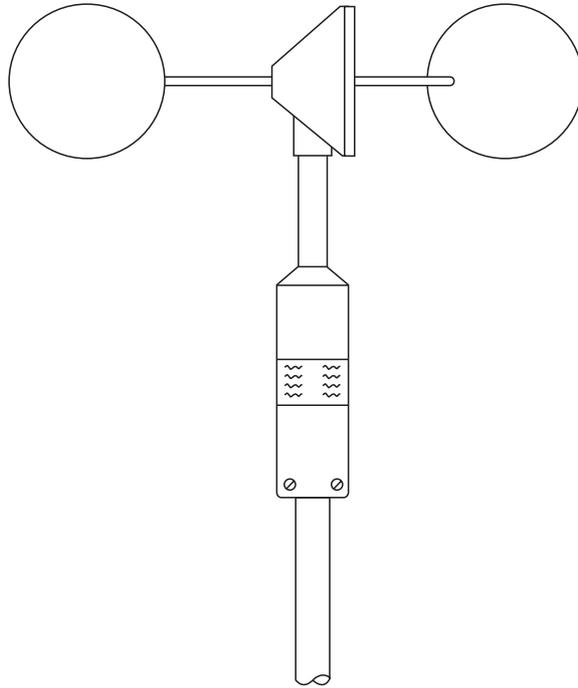
**Fig. 1.81** Three cup-anemometer.
