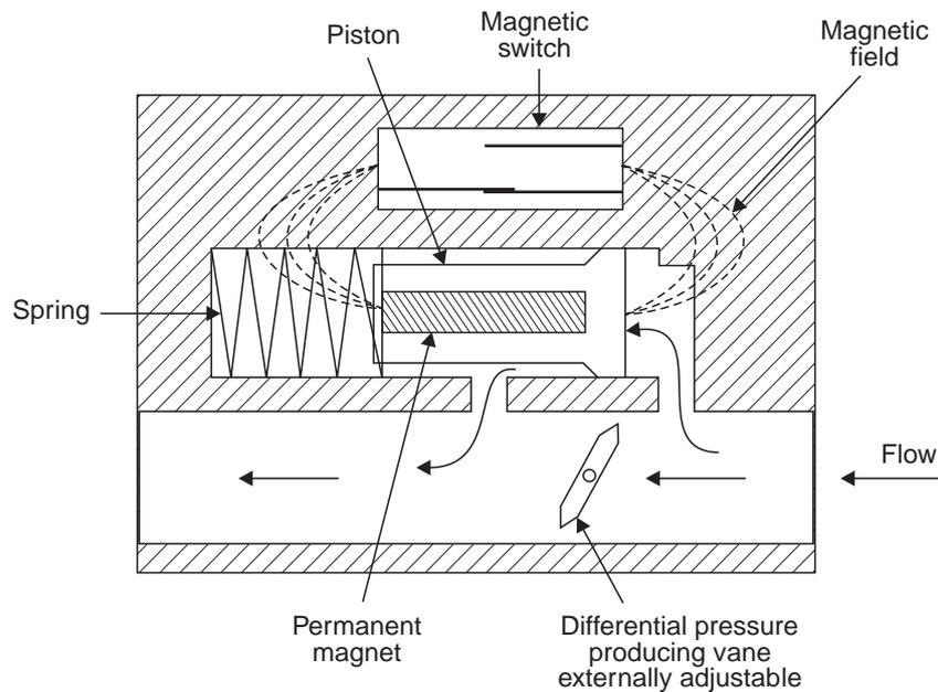
**Fig. 1.76** Bypass flow switch
