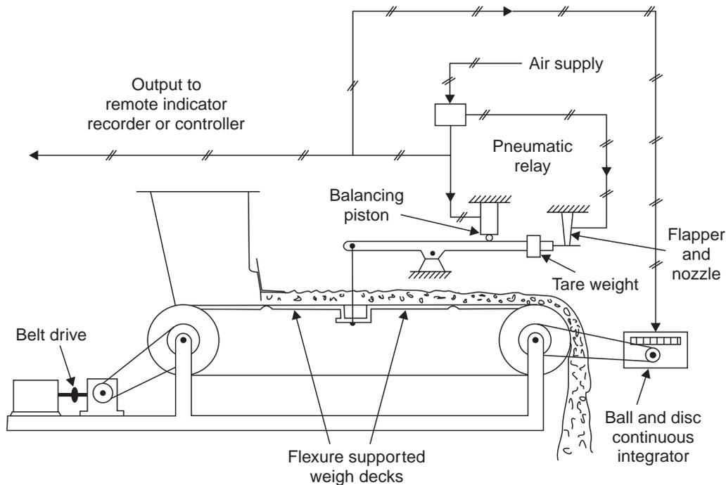
Fig. 1.68 Belt-type gravimetric meter with pneumatic system
