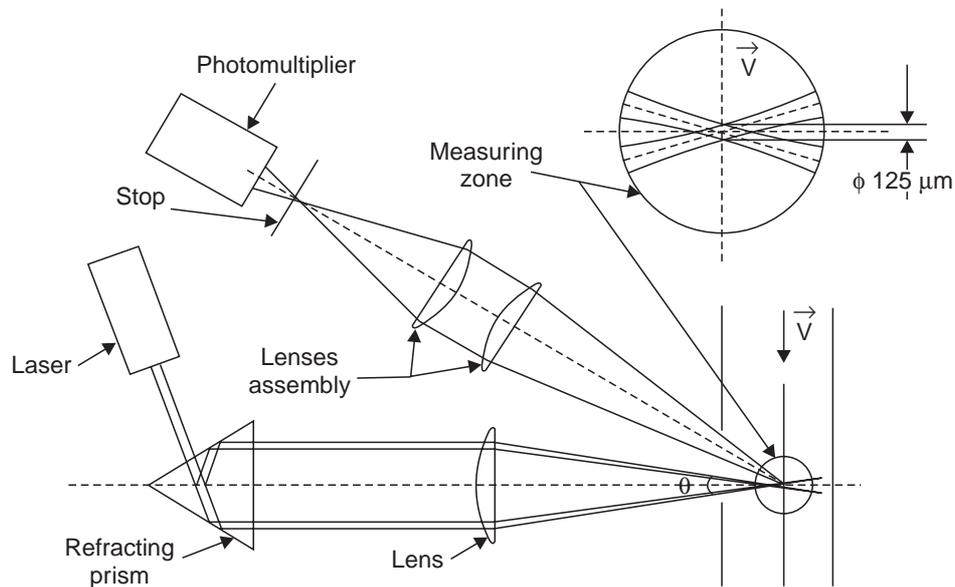
Fig. 1.61 Operation of the laser Doppler anemometer
