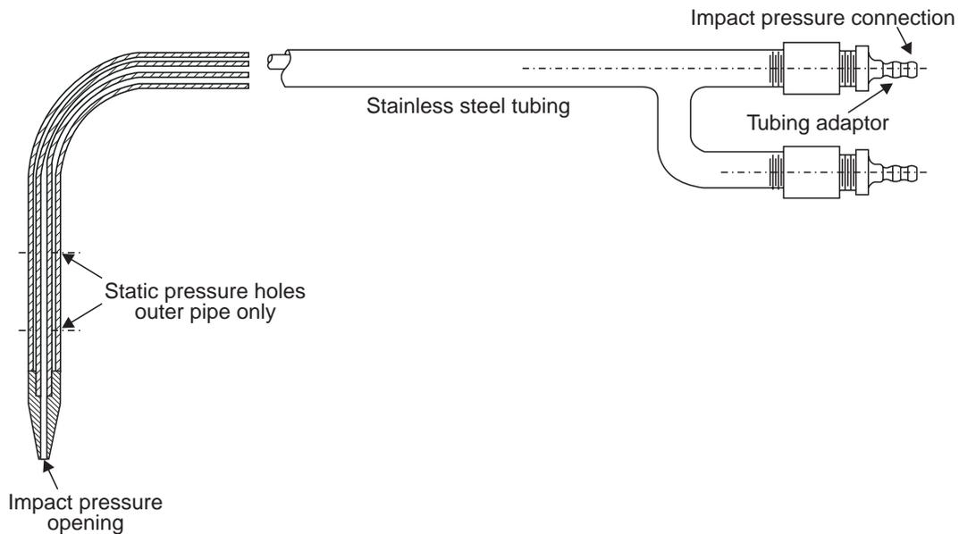
**Fig. 1.22** Typical pitot tube
