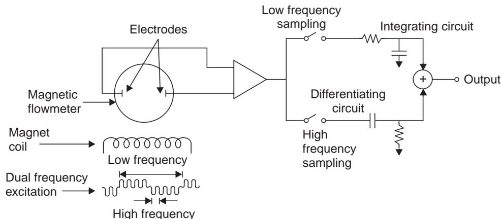
Fig. 1.55 Dual-frequency excitation Design
