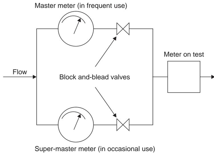
**Fig. 1.86** The use of two Master meters in alternate parallel
