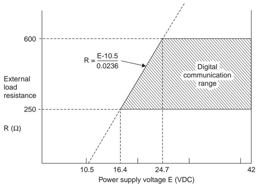
**Fig. 1.27** Relationship between power supply voltage and external load resistance
