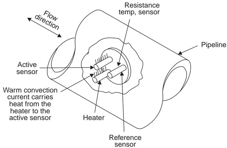
**Fig. 1.75** Thermal flow switch
