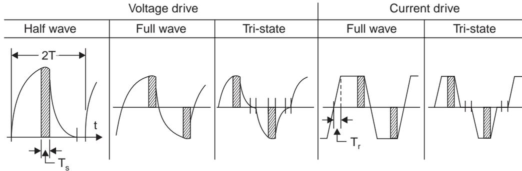
Fig. 1.53 Types of pulsed DC Coil excitation
