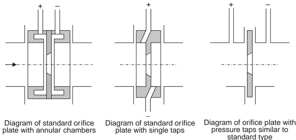
Fig. 1.6 Location of Pressure taps with Orifice plate
