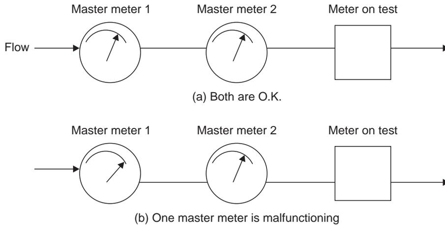
**Fig. 1.85** Two master meters are in series
