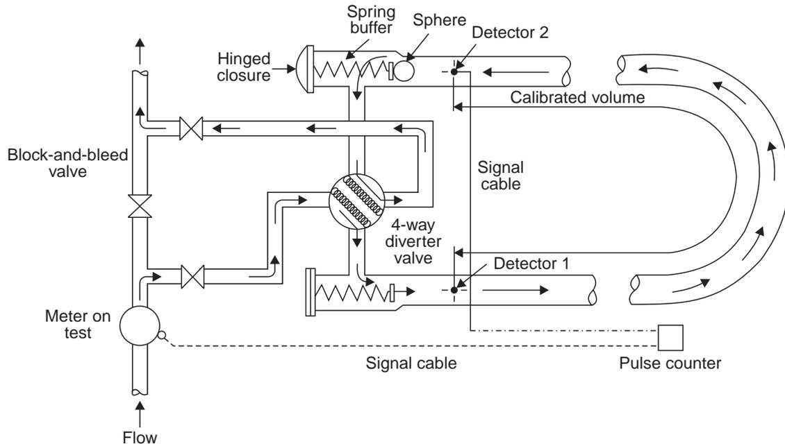
**Fig. 1.84** Principle of the bidirectional pipe prover
