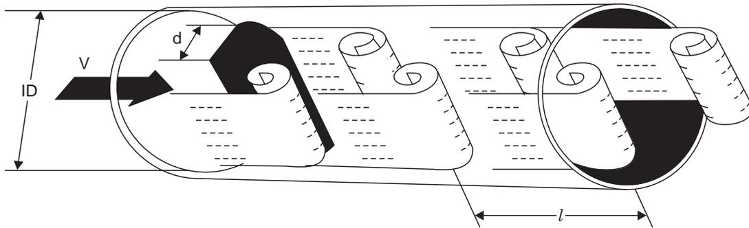
The distance between the Karman vortices ( $l$ ) is only a function of the width of the obstruction ( $d$ ) and therefore the number of vortices per unit of time gives flow velocity ( $V$ ).
