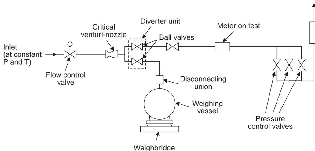
**Fig. 1.90** Simplified Arrangement of a Gravimetric system for compressed gases
