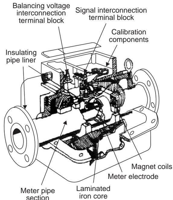
Fig. 1.56 Cutaway view of Electromagnetic flow meter
