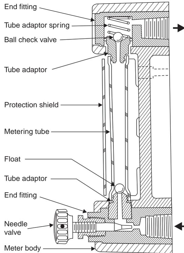
**Fig. 1.62** Purge rotameter with integral needle control valve
