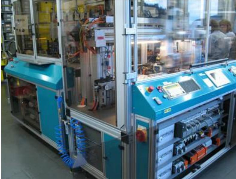
A manufacturer of limit switches upgraded to a multi-function safety relay system for its production cell to accommodate increased automation of the processes used in the construction of its products (Figure 3). The original safety circuit design was mostly manual, and thus required substantial operator interaction. The circuit had an E-stop, one set of safety light curtains, and door switches.
