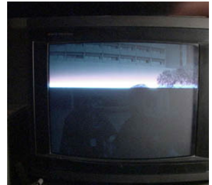
CRT in the middle of creating an image (showing scan line)
