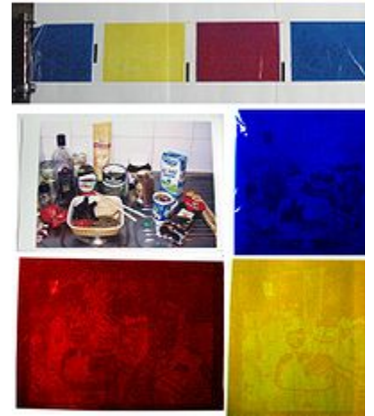
RGB dye sublimation panels before and after use showing wasted dye and potential privacy problems
