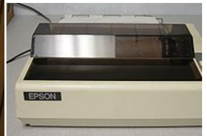
Epson MX-80 dot matrix printer – impact printers are still used for carbon copies
