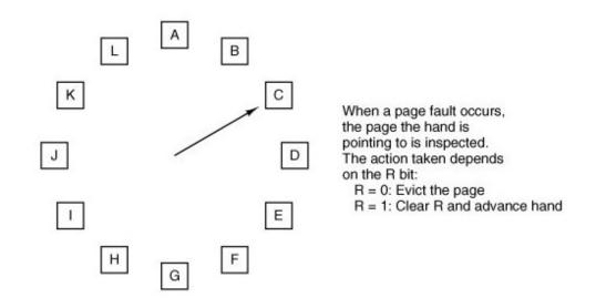
When a page fault occurs, the page being pointed to by the hand is inspected. If its R bit is 0, the page is evicted, the new page is inserted into the clock in its place, and the hand is advanced one position. If R is 1, it is cleared and the hand is advanced to the next page. This process is repeated until a page is found with R = 0
