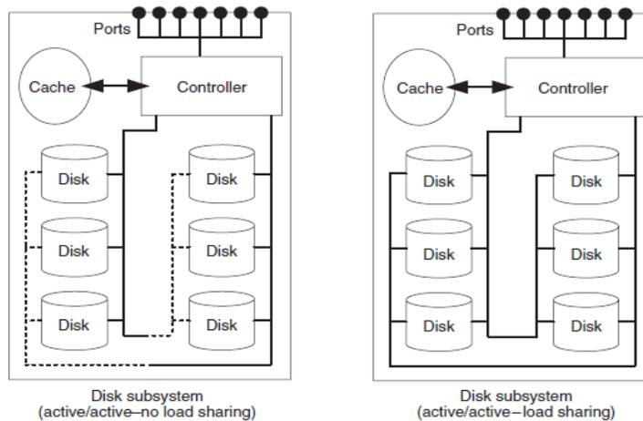
**Figure 2.6** Active/active cabling (no load sharing) uses both I/O channels at the same time. However, each disk is addressed via one I/O channel only, switching to the other channel in the event of a fault. In active/active cabling (load sharing) hard disks are addressed via both I/O channels.
