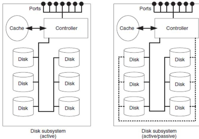
**Figure 2.5** In active cabling all hard disks are connected by just one I/O channel. In active/passive cabling all hard disks are additionally connected by a second I/O channel. If the primary I/O channel fails, the disk subsystem switches to the second I/O channel.
