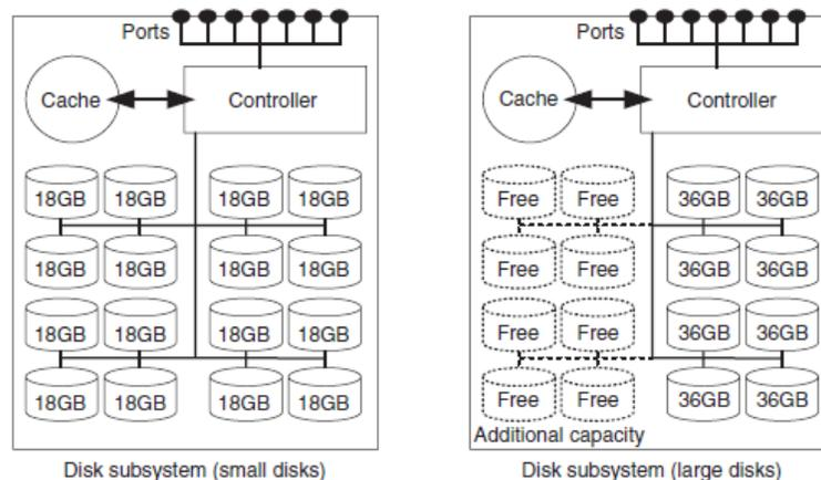
**Figure 2.4** If small internal hard disks are used, the load is distributed over more hard disks and thus over more read and write heads. On the other hand, the maximum storage capacity is reduced, since in both disk subsystems only 16 hard disks can be fitted.
