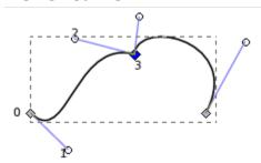
This Bezier curve shown has two segments, where each segment is defined by 4 control points. The curve interpolates two points and approximates the other two. The curve is defined by a Bernstein
