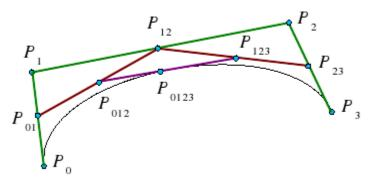
To calculate the point halfway on the curve, that is t=0.5 using De Casteljau's algorithm we (as shown above) find the midpoints on each of the lines shown in green, then join the midpoints of the lines shown in red, then the midpoint of the resulting line is a point on the curve. To find the points for
