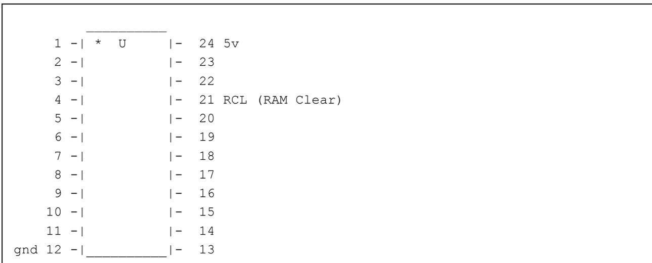
**NOTE:** Although these are 24-pin chips, the Dallas chips may be missing 5 pins, these are unused pins.
