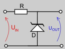
In the circuit shown, resistor R provides the voltage drop between  $U_{IN}$  and  $U_{OUT}$ . The value of R must satisfy two conditions:
