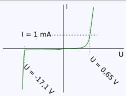
Current-voltage characteristic of a Zener diode with a breakdown voltage of 17 volt. Notice the change of voltage scale between the forward biased (positive) direction and the reverse biased (negative) direction.
