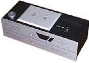
Top-loading CD player and external digital-to-analog converter.
