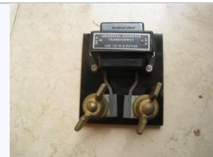
Transformer used for measuring higher ranges of AC current - 60A and 240A. Connected in series with circuit to be tested.
