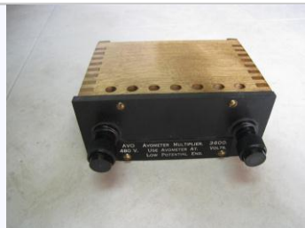
Multiplier for measuring higher ranges of AC and DC voltage up to 3600v.
