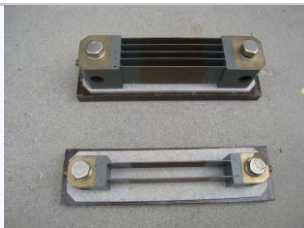
Shunts for measuring higher ranges of DC current - 480A and 120A. Connected in series with circuit to be tested.
