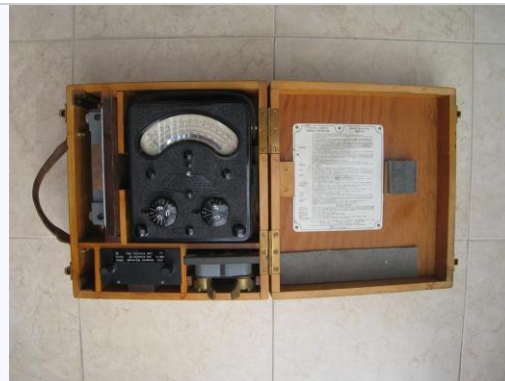
Avometer 48A in open wooden smart box including multiplier, transformer, two shunts, leads and prods.
