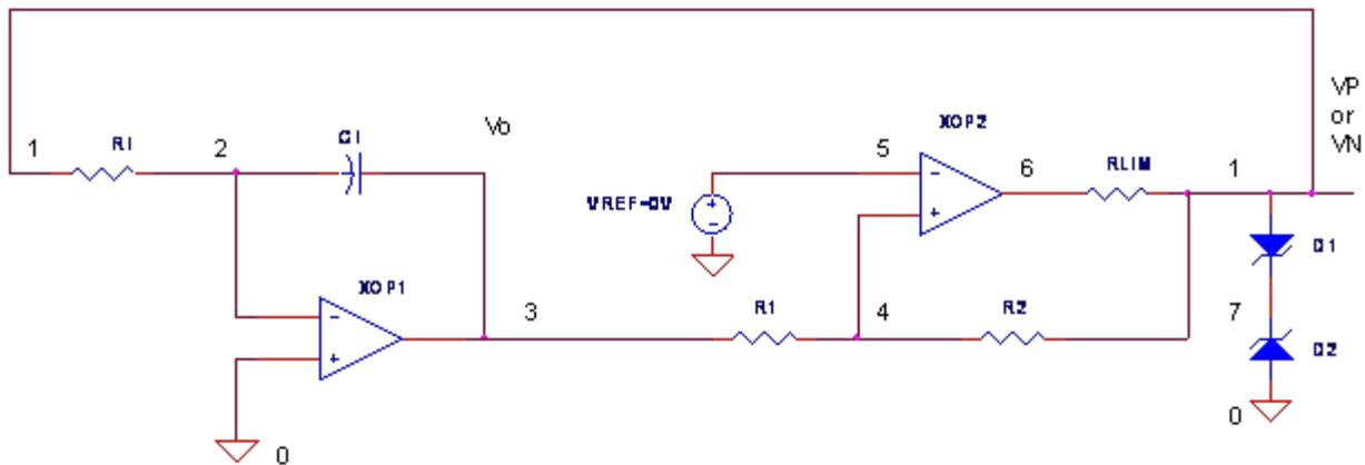
You may have noticed that the triangle peaks and period may not accurately meet our +/-10V swing at 100  $\mu$ s. The main reason is that our current source and thresholds are derived from zener diodes - not exactly the most accurate reference. Some designs use improved means for deriving and switching the current sources that charge CI.
