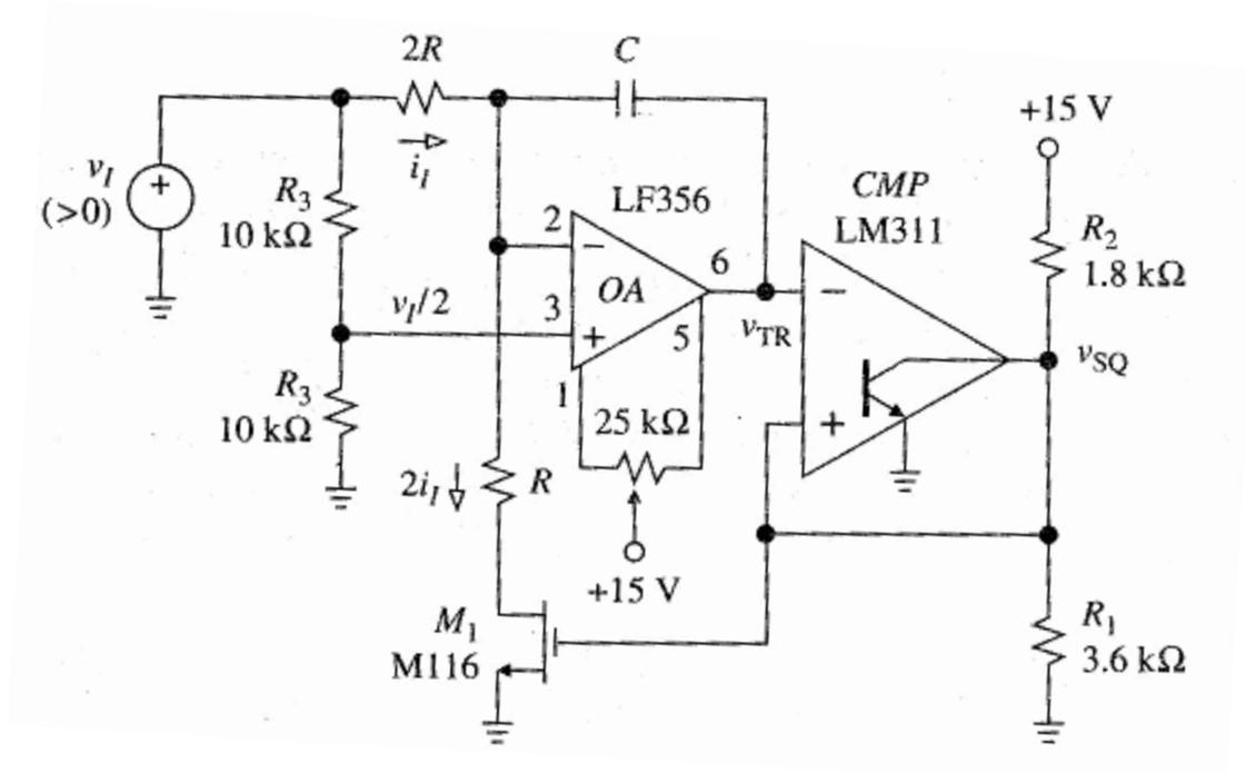
This signal generator gives you two waveforms for the price of one: a triangle-wave and a square-wave. The central component of this circuit is the integrator capacitor  $C$ . Basically we are interested in performing two functions on  $C$ : *charge it, discharge it - repeat indefinitely*. The output waveforms are shown here and it is apparent that a square wave generator followed by an integrator acts as a triangular wave generator.
