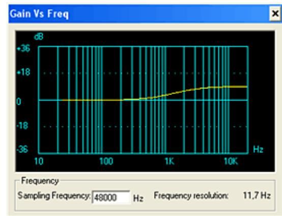
frequency is defined as the point where the gain is  $\pm 3$  dB from the horizontal section, it depends on the roll-off rate. The picture at the right has the same settings as the previous picture, except that the treble gain is at +9 dB.
