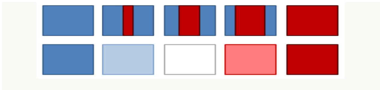
The two switching mechanism in a ferroelectric: domain-based (top) and without domains (bottom).
