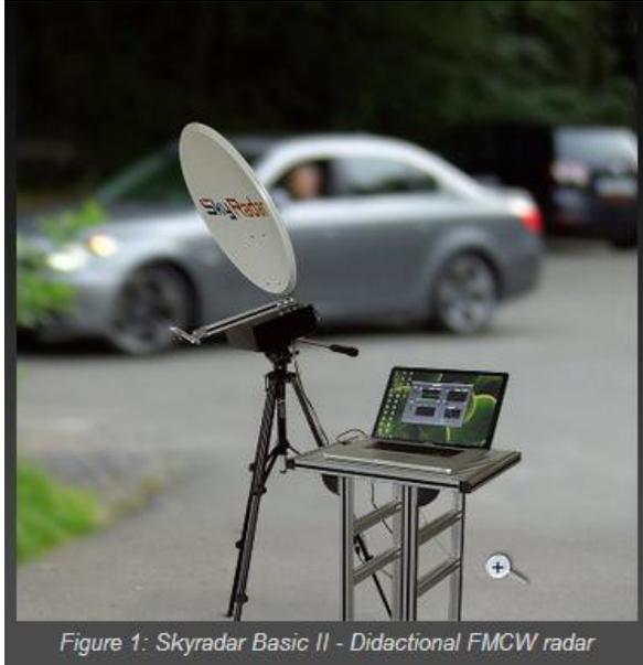
Figure 1: Sky radar Basic II - Didactical FMCW radar
