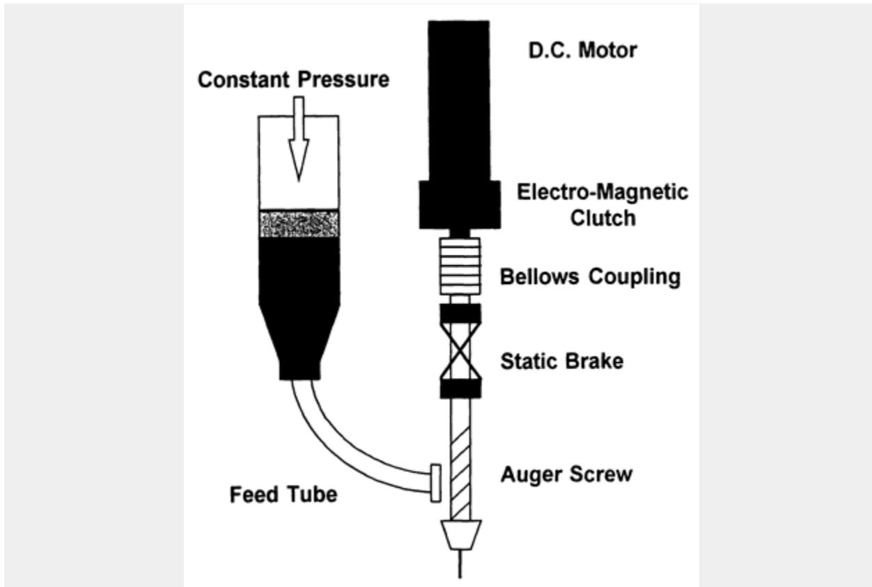
The available needle pressure is higher (>250psi) than with the syringe (90psi), reducing the possibility of clogging, and there is at least the potential (if time allows) for the screw to be reversed at the end of its stroke to relieve the pressure and provide a clean cut-off without weeping.
