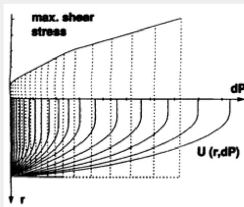
Steady-state flow of a viscous incompressible fluid in a tube, showing the radial variation of the velocity profile
