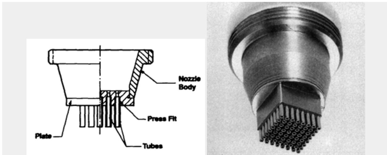
The nozzle has to supply the required volume of adhesive in one 'shot', to provide a void-free bond line, of the right thickness, and with the right amount of filleting. The number of tubes is determined by the size of the chip, the bond line thickness, and the volume dispensed by each tube. A rule of thumb suggested by Sela to give a bond-line thickness of 40 $\mu$ m is
