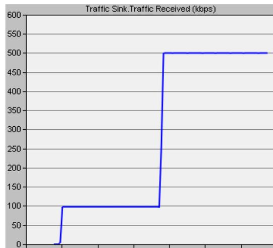
Figure 4. Handover from GPRS to UMTS (FTP)
