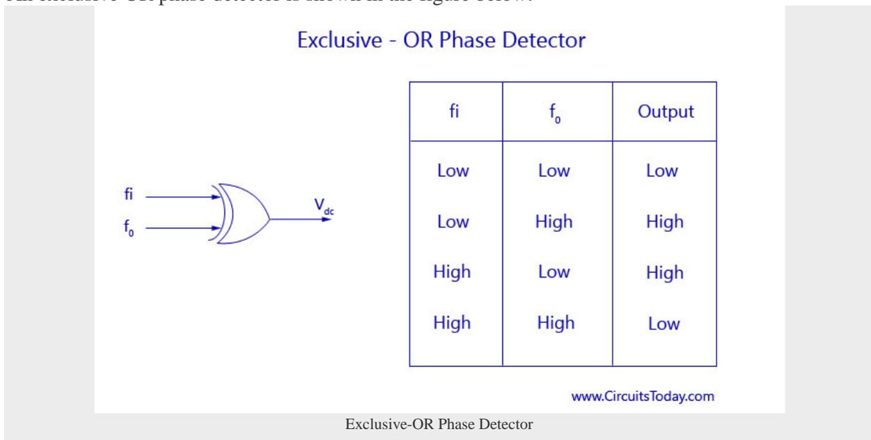
It is obtained as a CMOS IC of type 4070. Both the frequencies are provided as an input to the EX OR phase detector. Obeying the EX-OR concept the output becomes HIGH only if either of the inputs  $f_i$  or  $f_o$  becomes HIGH. All other conditions will produce a LOW output. Let us consider a waveform where the input frequency leads the output frequency by  $\theta$  degrees. That is,  $f_i$  and  $f_o$  has a
