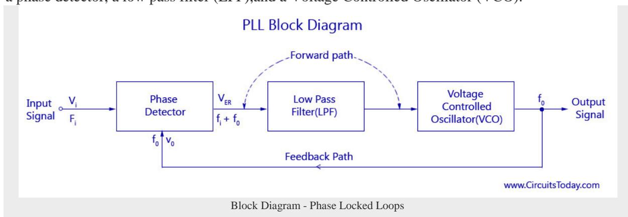
Block Diagram - Phase Locked Loops
