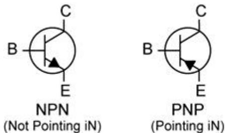
**Ohmmeters view of the BJT.** Clearly a transistor cannot be made on the bench by combining two diodes. (Why is that?) Most ohmmeters cannot only measure the resistance, but also measure the forward voltage drop across a diode. From this perspective you can identify the base and the type of transistor based on the following equivalent circuits.
