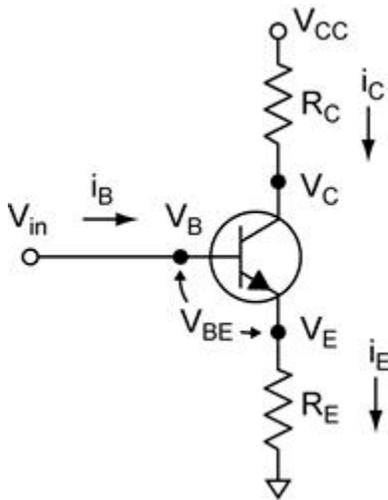
Impedance is defined as  $Z = V/I$ . In linear circuits (with resistors, capacitors, inductors, batteries, etc.) this ratio is the reciprocal of the slope of the  $I$  versus  $V$  graph. In circuits with nonlinear elements such as a transistor, the input impedance of the transistor is defined as the reciprocal of the slope of the  $I$  versus  $V$  graph. This is simply the derivative of  $V_{in}$  with respect to  $I_{in}$ .
