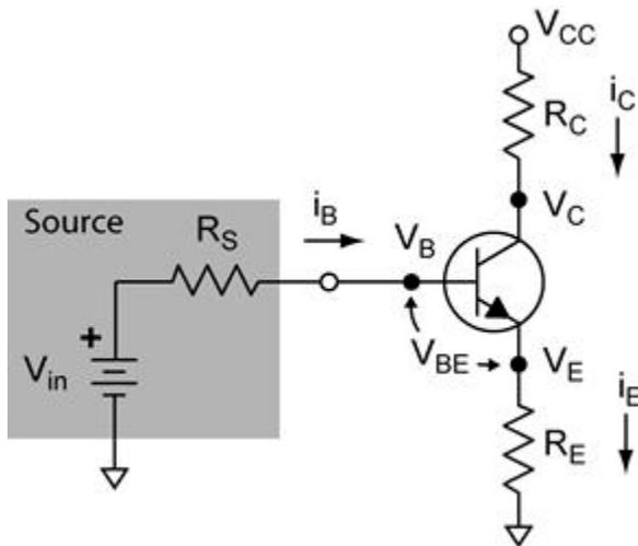
The output impedance seen by the load ( $R_E$  in this example) is defined as:
