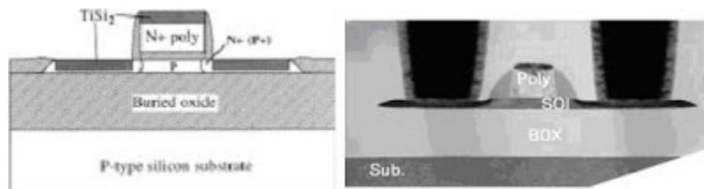
**Figure (3) Cross section of an n (p)-channel thin-film SOI MOSFET [1]**
