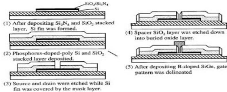
**Figure (2) FinFET process flow steps [2]**
