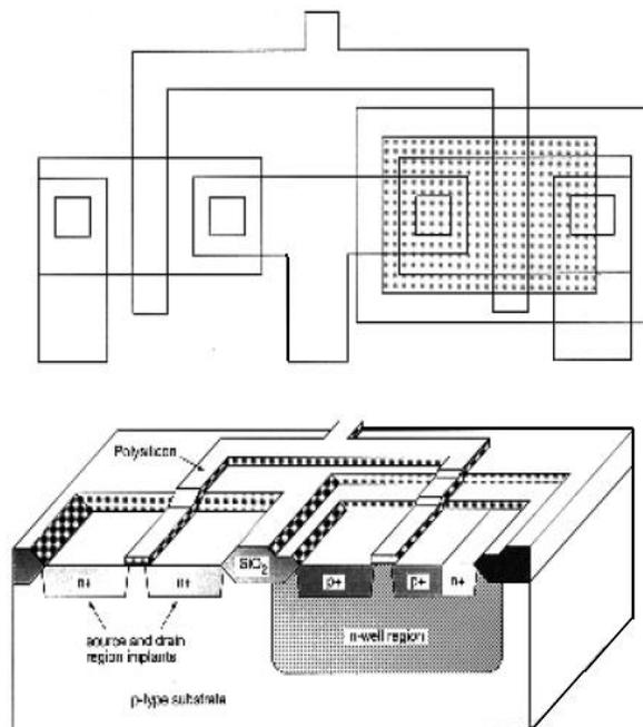
Figure-11.3: Using a set of two masks, the n+ and p+ regions are implanted into the substrate and into the n- well, respectively. Also, the ohmic contacts to the substrate and to the n-well are implanted in this process step.
