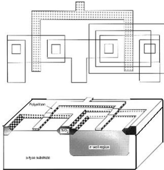
Figure-11.2: Cross sectional view
