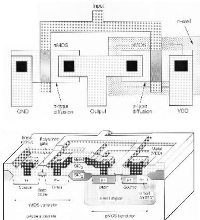
Figure-11.6: The composite layout and the resulting cross-sectional view of the chip, showing one nMOS and one pMOS transistor (built-in n-well), the polysilicon and metal interconnections. The final step is to deposit the passivation layer (for protection) over the chip, except for wire-bonding pad areas.
