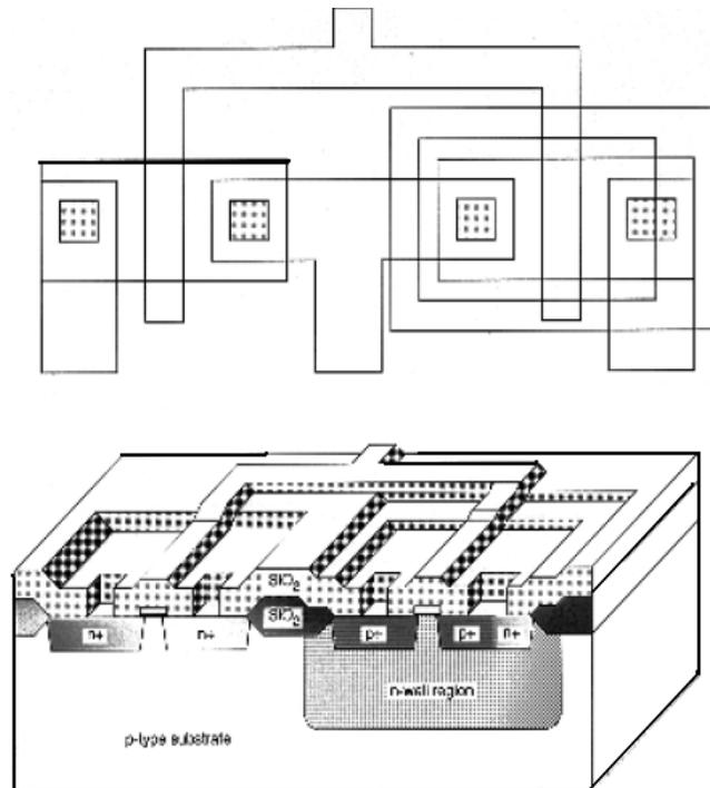
Figure-11.4: An insulating silicon dioxide layer is deposited over the entire wafer using CVD. Then, the contacts are defined and etched away to expose the silicon or polysilicon contact windows. These contact windows are necessary to complete the circuit interconnections using the metal layer, which is patterned in the next step.
