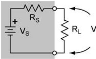
$$0 = \frac{dP_L}{dR_L} \quad P_L = \frac{V^2}{R_L} \quad V = V_S \left( \frac{R_L}{R_S + R_L} \right)$$
