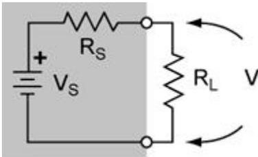
$$0 = \frac{dP_L}{dR_S} \quad P_L = \frac{V^2}{R_L} \quad V = V_S \left( \frac{R_L}{R_S + R_L} \right)$$
