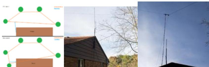
After adding a fifth anchor point the loop is now a distorted pentagon instead of trapezoidal in shape (see the sketch for the rough layouts).
