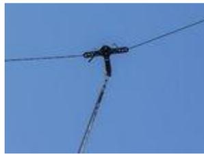
The feedline I chose is 300 ohm ladder line, which is a little harder to find than its 450 ohm cousin. Some ladder line is cheaply made, but this type from DX Engineering uses 18 AWG copper-clad steel and works very well. They also make a great antenna feed point kit with built in strain relief slots for use with their 300 ohm ladder line. It is well worth the money.
