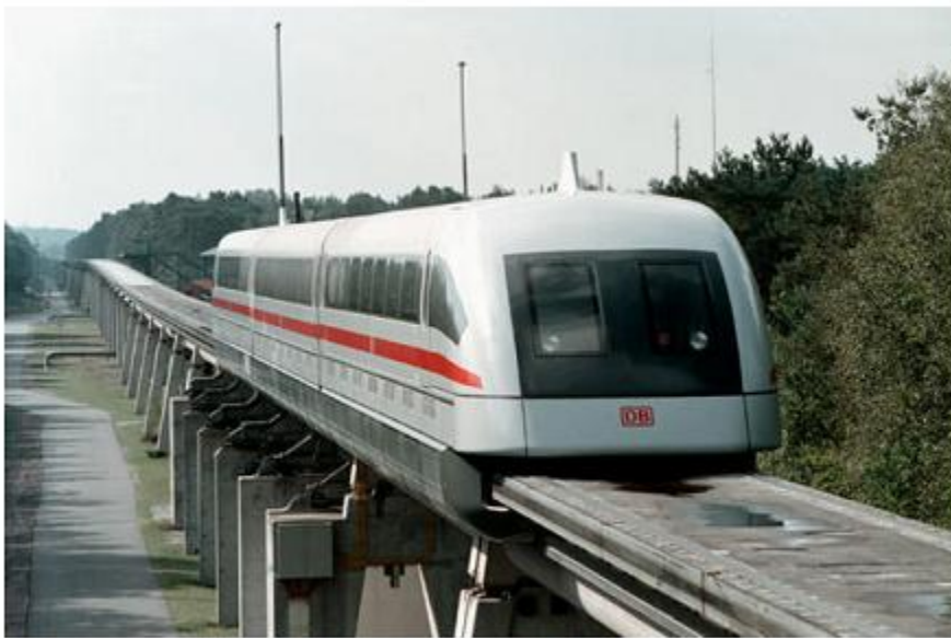
Fig. 256: high speed vehicle Transrapid 08 , testing site Emsland, Germany (source: Thyssen)
