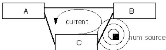
But, if A is connected to B which is connected to C which is connected back to A, there's a circular path in the shields through which current will flow with the slightest encouragement. Encouragement can come from lots of things, such as those stupid power transformers blocking most of the holes in the power strips. It wouldn't be much of a studio without some complex patching, so here's how to minimize the damage:
