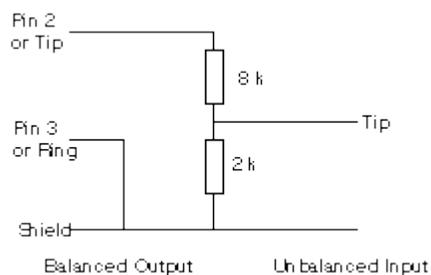
Some equipment does not take kindly to being unbalanced in this way. The frequency response is messed up by shorting one of the output pins to the shield. This happens mostly with vintage gear, especially tube circuits. In that case you must use an impedance matching transformer to connect it to unbalanced inputs.
