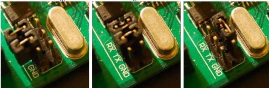
In the picture, from left to right: TTL UART, RS485 and loopback jumper configurations. In TTL mode, TX and RX pins are the one on the crystal side with the pinout indicated in the silkscreen.
