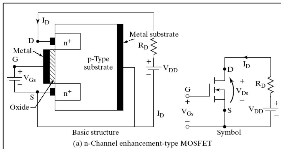
Fig. 2.17: Structure of n-channel enhancement type MOSFET
