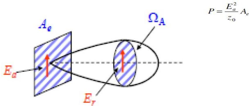
Assuming a uniform field  $E_r$  in far field at a distance  $r$ , Power Radiated is also given by  $P = \frac{E_r^2}{z_0} r^2 \Omega_A$
