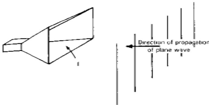
Let the poynting vector or power density of the plane wave be  $S$  watts/sq -m and let the area or physical aperture be  $A_p$  sq-m. If the Horn extracts all the power from the Wave over it's entire physical Aperture  $A_p$ , Power absorbed is given by  $P=SA_p= (E^2/Z)A_p$  Watts,  $S$  is poynting vector ,
