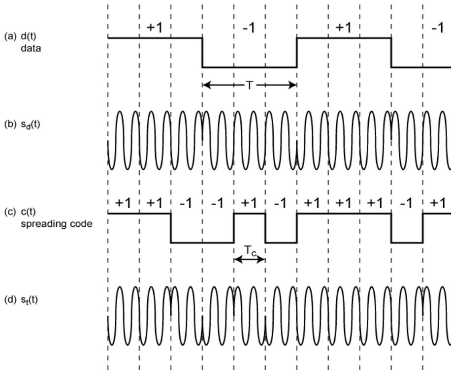
Direct Sequence Spread Spectrum Using BPSK Example
