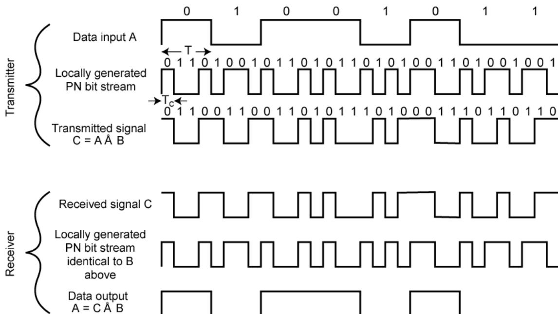
Direct Sequence Spread Spectrum Transmitter/receiver:
