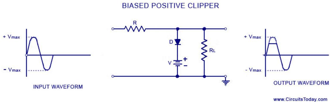
Some of other biased clipper circuits are given below in the figure. While drawing the wave-shape of the output basic principle discussed above are followed. The diode has been considered as an ideal one.
