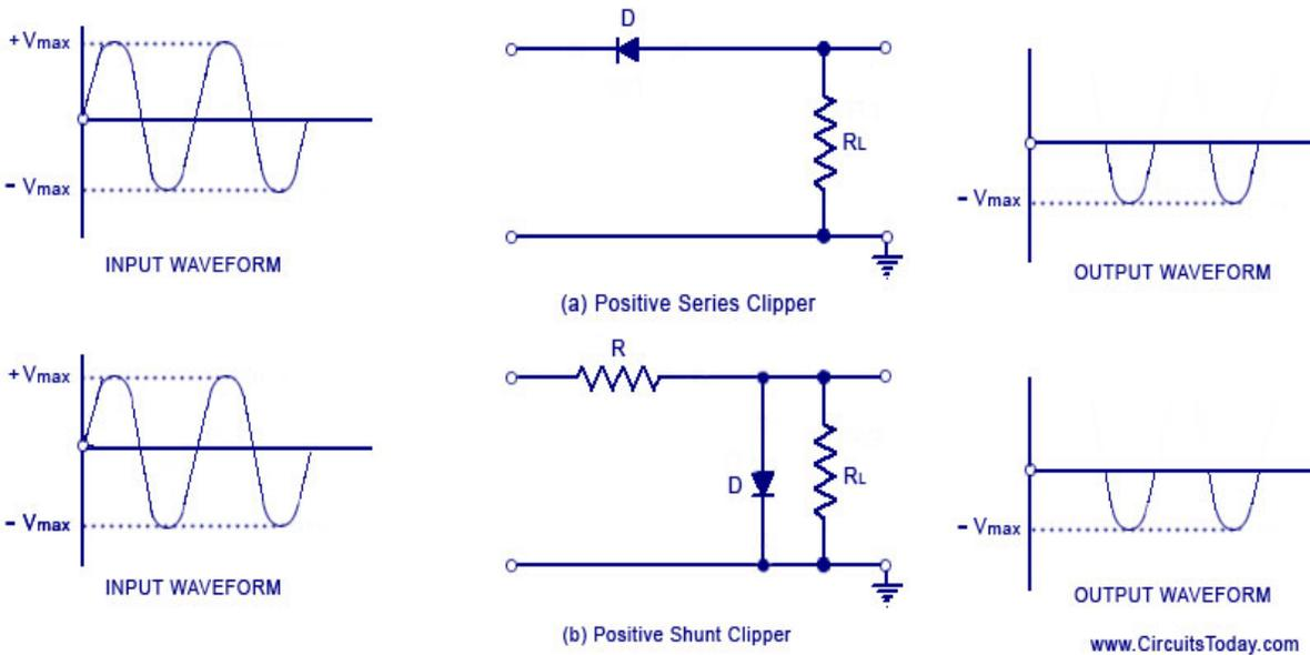
As shown in the figure, the diode is kept in series with the load. During the positive half cycle of the input waveform, the diode 'D' is reverse biased, which maintains the output voltage at 0 Volts. Thus causes the positive half cycle to be clipped off. During the negative half cycle of the input, the diode is forward biased and so the negative half cycle appears across the output.
