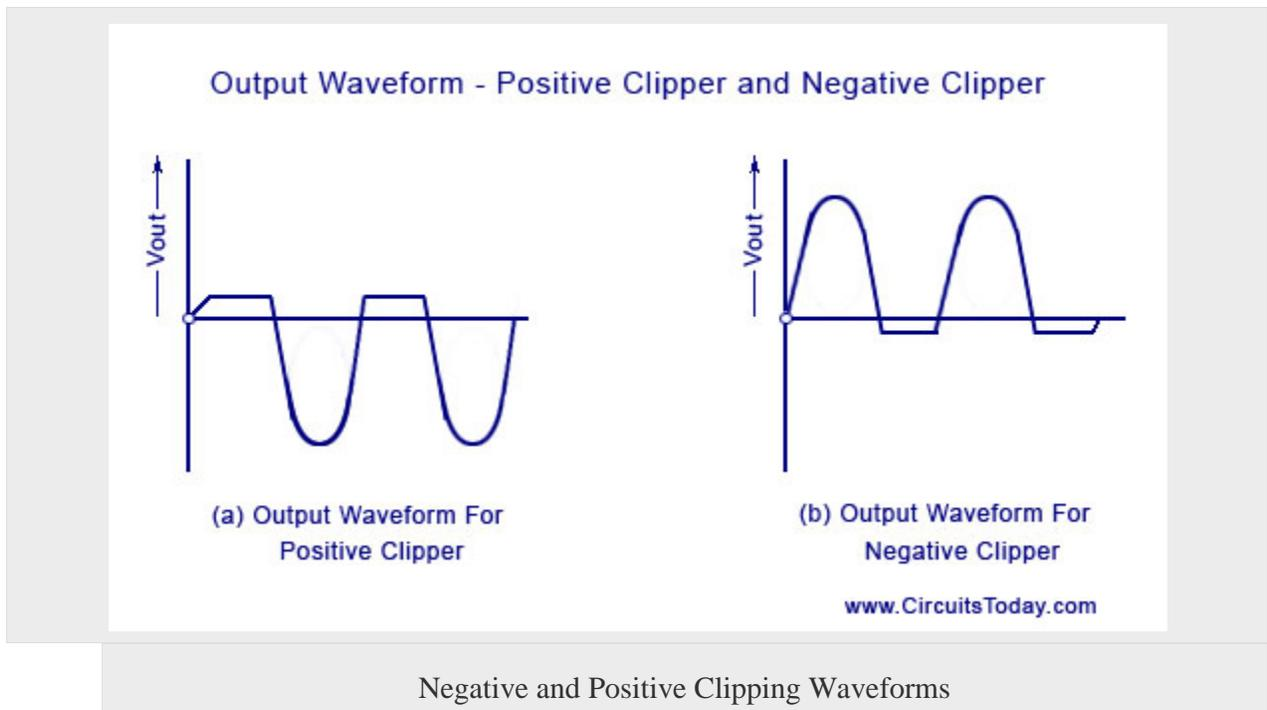
Negative and Positive Clipping Waveforms
