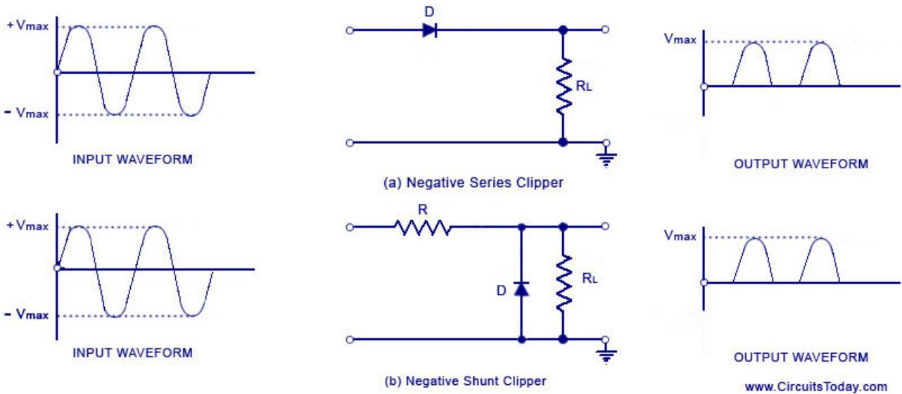
In all the above discussions, the diode is considered to be ideal one. In a practical diode, the breakdown voltage will exist (0.7 V for silicon and 0.3 V for Germanium). When this is taken into account, the output waveforms for positive and negative clippers will be of the shape shown in the figure below.
