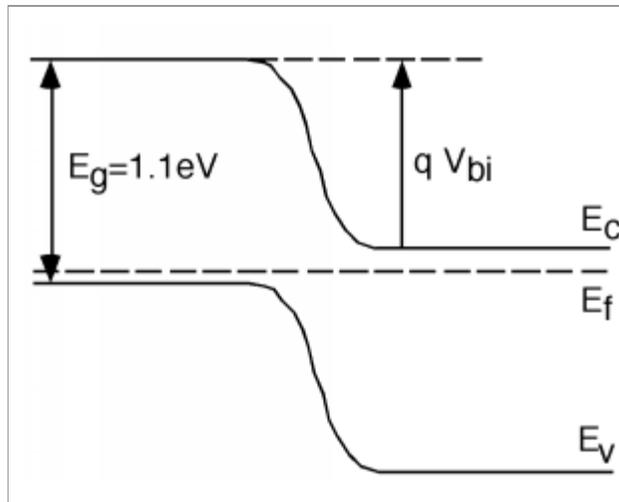
**Figure 3:** Band diagram for a p-n junction
