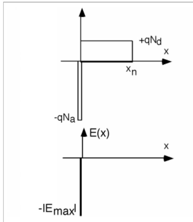
**Figure 1:** Finding the electric field in the p-type region
