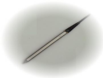
Obviously, the electronics of these interfaces add to the price of the bar-code reader. The RS232 interface furthermore requires external power. A low cost option, is to use a *bar-code wand*—a pen-style reader. If the H0420 MP3 controller is programmed to understand the pulse train produced by a wand, no decoder or emulation interface is needed. Such "undecoded" wands are in the price range of \$50.= to \$100.= for rugged, steel-housed pens; a fraction of the price of a CCD or a LASER scanner.
