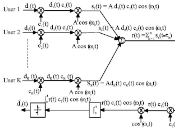
Block diagram of a simple asynchronous DS-SSM system
