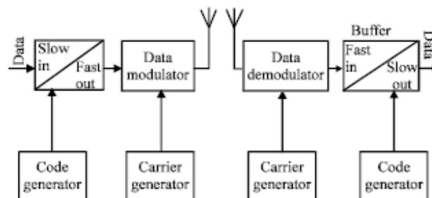
Block diagram of a TH-CDMA transmitter and receiver
