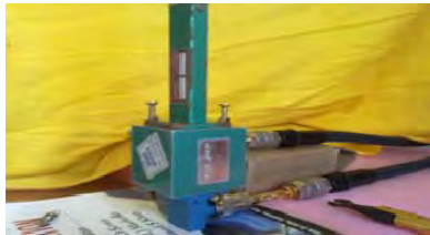
Fig 6.: Measurement setup for testing 3- port Circulator XC-621
