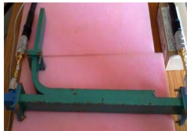
Fig 13:Measurement Setup for Directional coupler characteristics
