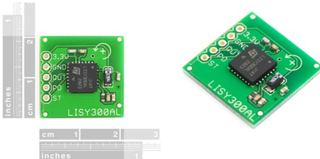
Fig 3.2 - Gyroscope with evaluation board
