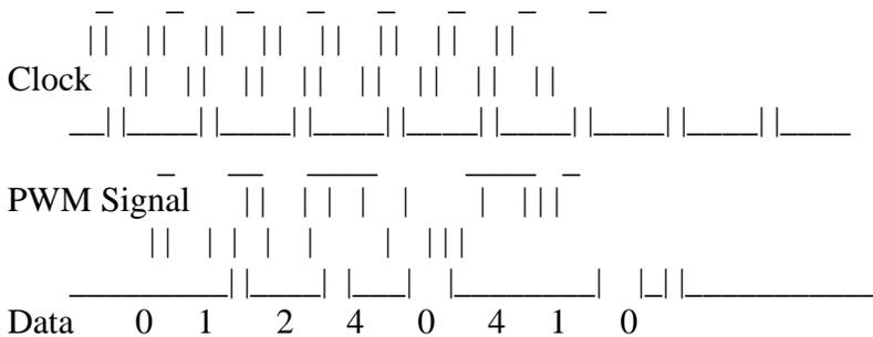
The inclusion of a clock signal is not necessary, as the leading edge of the data signal can be used as the clock if a small offset is added to the data value in order to avoid a data value with a zero length pulse.
