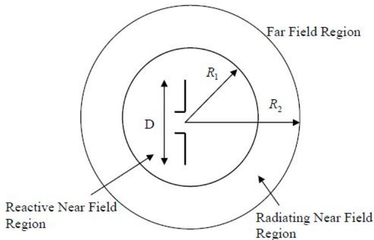
**Fig 2** Field regions around the antenna
