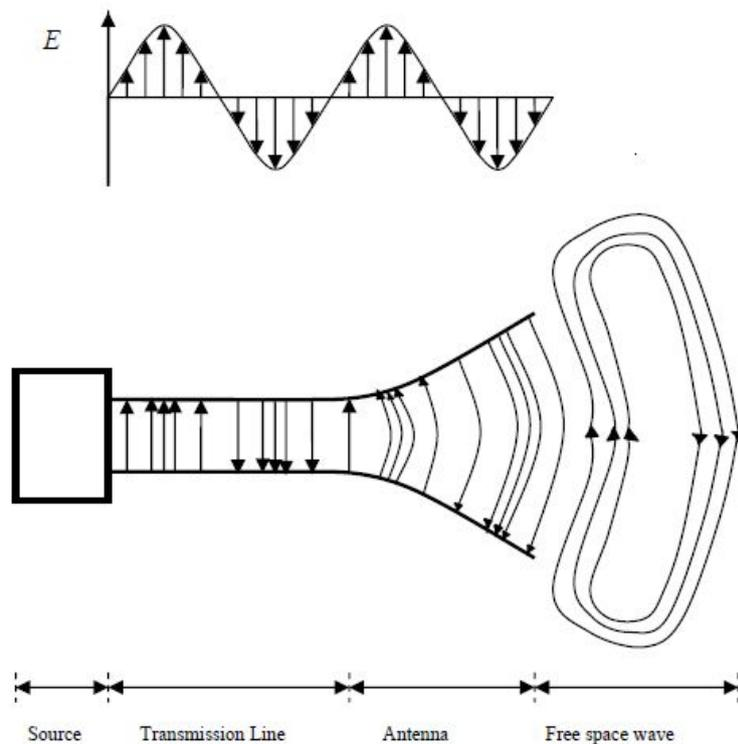
**Fig 1 Radiation from an antenna**
