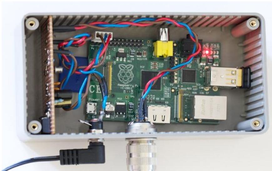
Interfacing the Raspberry Pi's serial output to the Nixie clock proved equally easy.
