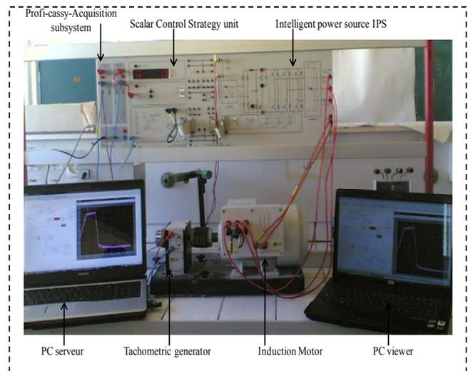
Fig. 5 A photo of the experimental set up
