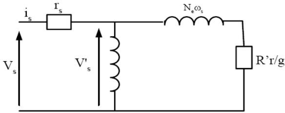
Fig. 4 Block diagram of the equivalent monophasic of the induction motor model
