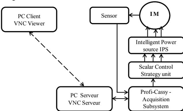
Fig. 3 Block diagram of the control design
