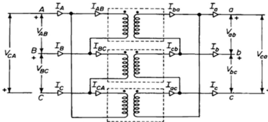
As clear from the figure, a three phase transformer will have three primary coils and three secondary coils. The manner, in which the three windings are connected with each other, can be a delta connection or a Y connection. Both of these are shown below:
