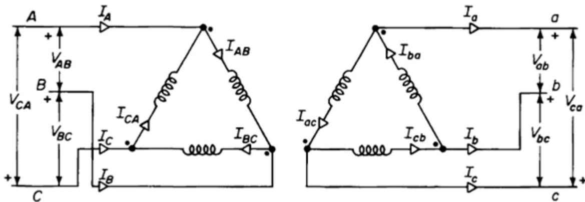
If the coils are connected in series, forming a closed loop, then the connection is known as a delta connection, but if the three windings are connected such that all have a common point then a Y-type connection is formed. It has a neutral wire at the common end point. Both of these connections are equivalent and are inter convertible from one form to another.
