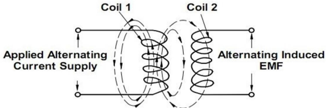
These windings are usually made on an iron core to make the magnetic field stronger, and laminated afterwards, so that the flux does not weaken due to air, which is a perfect insulator. But still some power losses are observed such as Eddy Current losses and Hysteresis loss.
