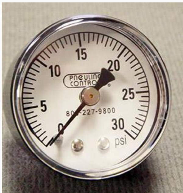
Transformer pressure gauge
