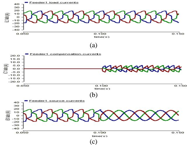
Fig. 8 Feeder1 currents: (a) load (b) compensation (c) source
