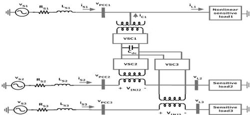
Fig. 2 Shunt and series compensators of GUPQC
