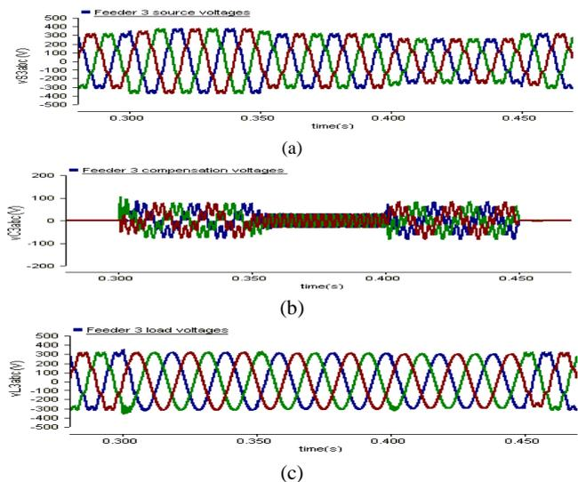
Fig. 12 Feeder3 voltages: (a) supply (b) compensation (c) load
