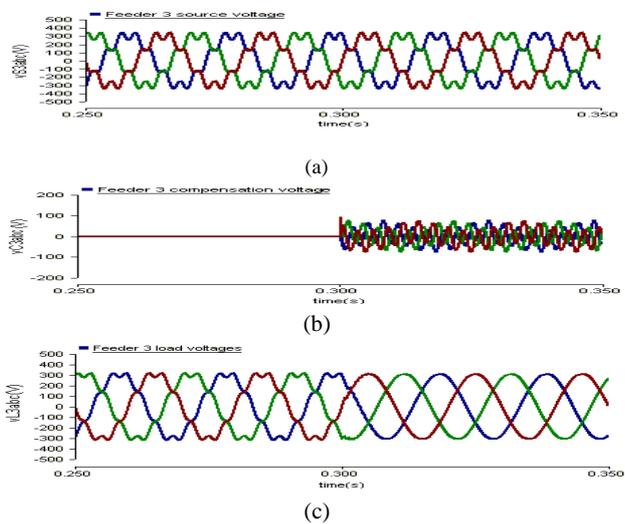
Fig. 10 Feeder3 voltages: (a) supply (b) compensation (c) load
