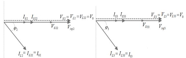
Fig. 7 Phasor representation of series compensators loading
