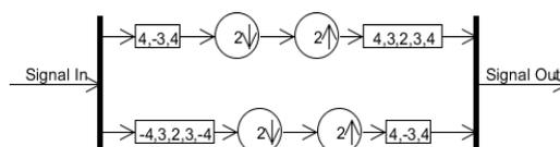
Figure 6. The biorthogonal filter bank
