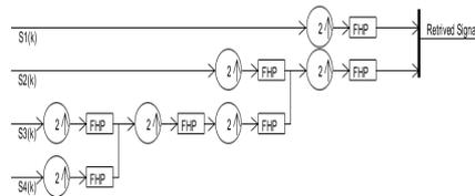
Figure 4. Inverse dyadic spectral transform realized with the tree structure of high-pass (FHP) and low-pass (FLP) retrieval filters. Note: The up-sampling operation  $\uparrow 2$  inserts zeros between the samples.
