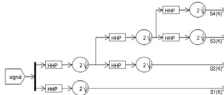
Figure 3. Dyadic spectral transform realized with the tree structure of high-pass (HHP) and low-pass (HLP) decomposition filters.
