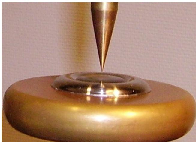
Figure 3. Water surface with the point electrode.
